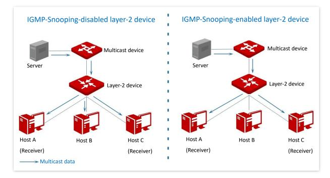
IGMP snooping only forwards data to the specific receivers through the layer-2 multicast, providing the following advantages:
