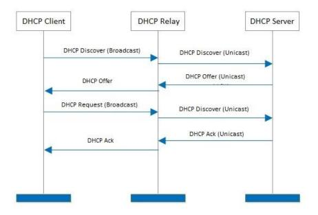
The working principles of DHCP Relay are shown below.
